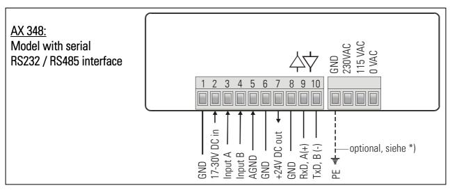
\*) The connection of PE is optional and not necessary for safety or for EMC. However, with some applications, it can be useful to ground the common potential of all signal lines
