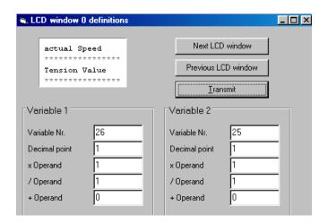
There are totally 4 LCD windows accessible (0 − 3) and the actual window number appears in the blue head line. To change from one window to another, use the keys "Next LCD window" or "Previous LCD window".
