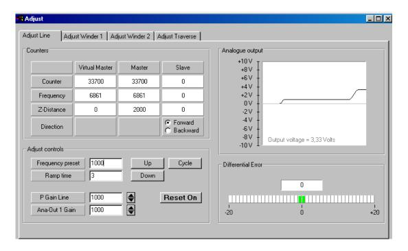
The Adjust Menu provides a choice between the drives "Line", Winder1", "Winder2" and "Traverse". You must only adjust the drives which are physically used with your application. The Adjust Program uses the virtual master axis and treats all drives as Slaves during the tuning process, independent of the later configuration and application. Only the drive which actually is selected will move, and all other drives remain in standstill.
