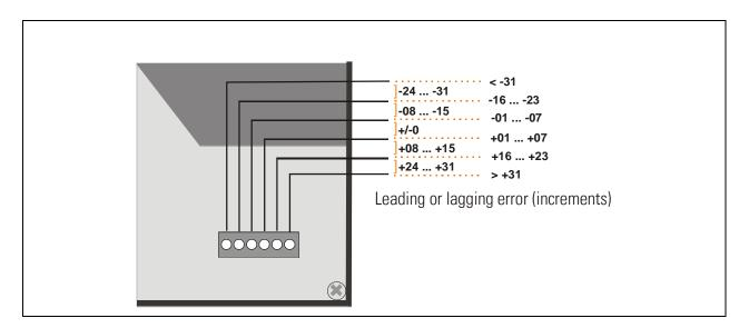
Positive errors (LEDs on right site of centre position) indicate that the drive lags the line. Negative errors (LEDs on left site of centre position) indicate that the drive leads the line. Under regular production conditions and with good adjustment of the control loop, you should find between 2 and 4 of the centre LEDs on or blinking, which indicates at the same time that the accuracy is fine.
