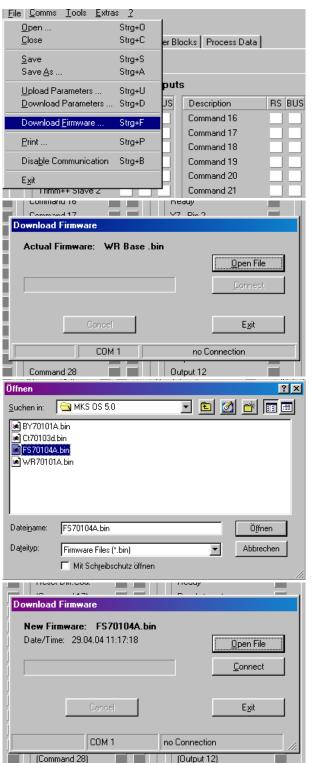
Connect the PC to the controller, using a RS232 cable (see 3.8 of the hardware manual). Apply power to the controller and start the OS5.1 PC software. Select "Download Firmware" from the "File" menu.
